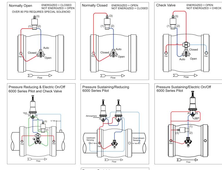
Pressure Sustaining 6000 Series Pilot and Check Valve
